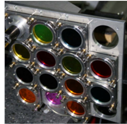
Filter matrix with 13 interference filters. Part of the Hellride Instrument.
